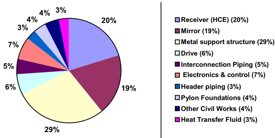
The S&L review focuses on these five major cost components: concentrator structure, mirrors, receivers, thermal energy storage, and the power block. Table 4-4 provides a summary of the SunLab and S&L cost projections for these five cost elements.
