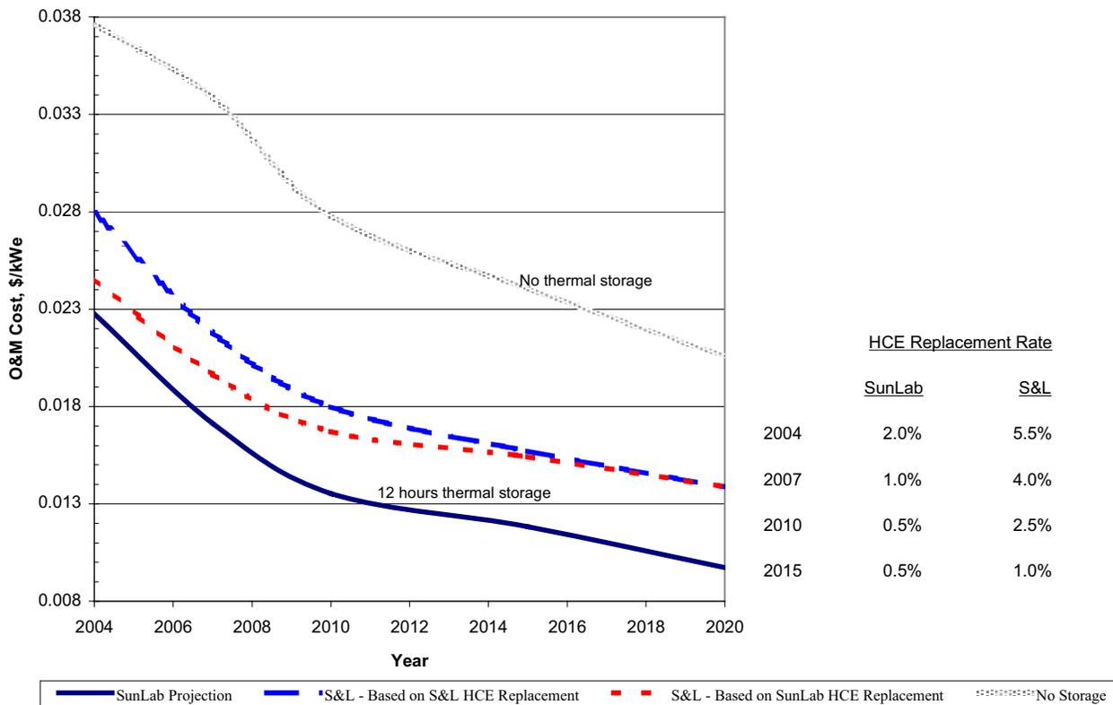
The reduction in O&M cost is primarily a result of the increase in plant size and the increase in annual plant capacity factor. The plant capacity increases directly as a result of the increases in thermal storage. Increasing the size (MWe) and capacity factor of the power plant incurs minimal increase in the fixed O&M expenses (\$/year).
