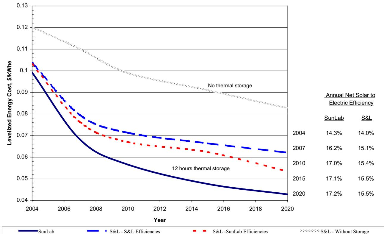
The curves highlight the impact of the annual net efficiencies on the levelized energy costs. The curves also indicate that additional cost reductions above and beyond the more conservative S&L values, due to technology improvements, reduced HCE replacement rates, and increased deployment rates, will result in further convergence of the levelized energy costs toward the projected SunLab values.
