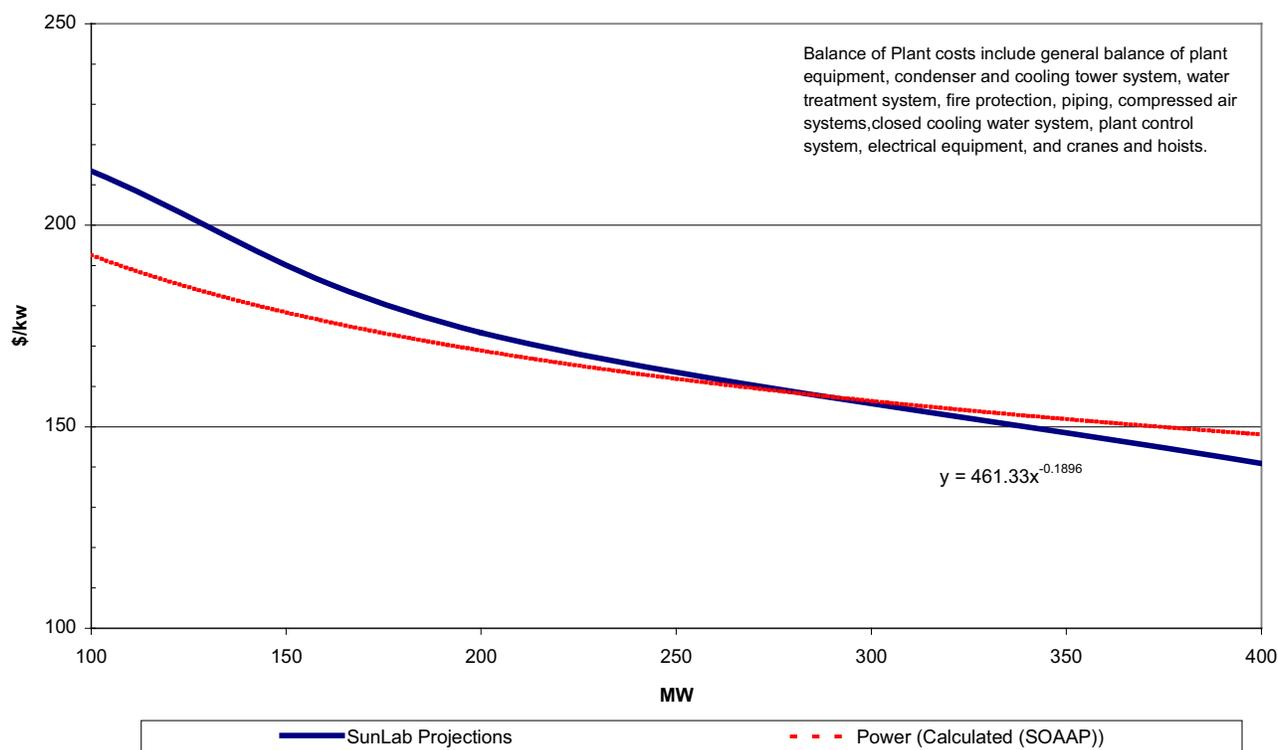
A comparison of the SunLab projected cost versus the SOAPP predicted \$/kW cost for the power block plus the balance-of-plant is shown in Table 4-10.
