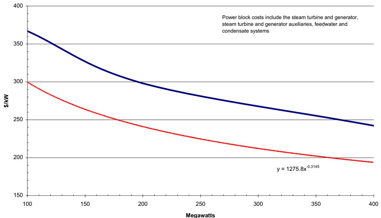
**Figure 4-3B — Scale-Up Cost Reductions: Balance-of-Plant (\$/kW)**
